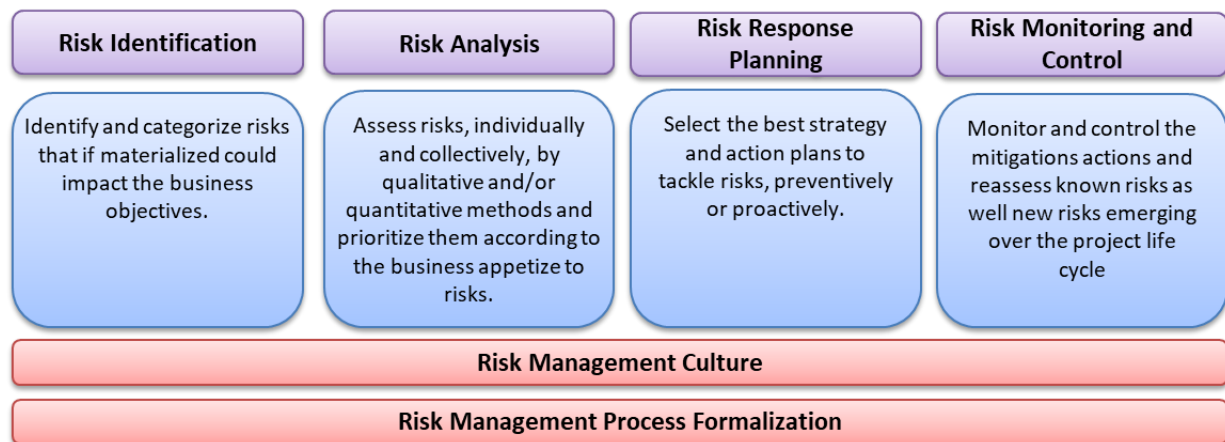
Figure 4. Common process of project risk management supported by risk management culture and by risk management process formalization
